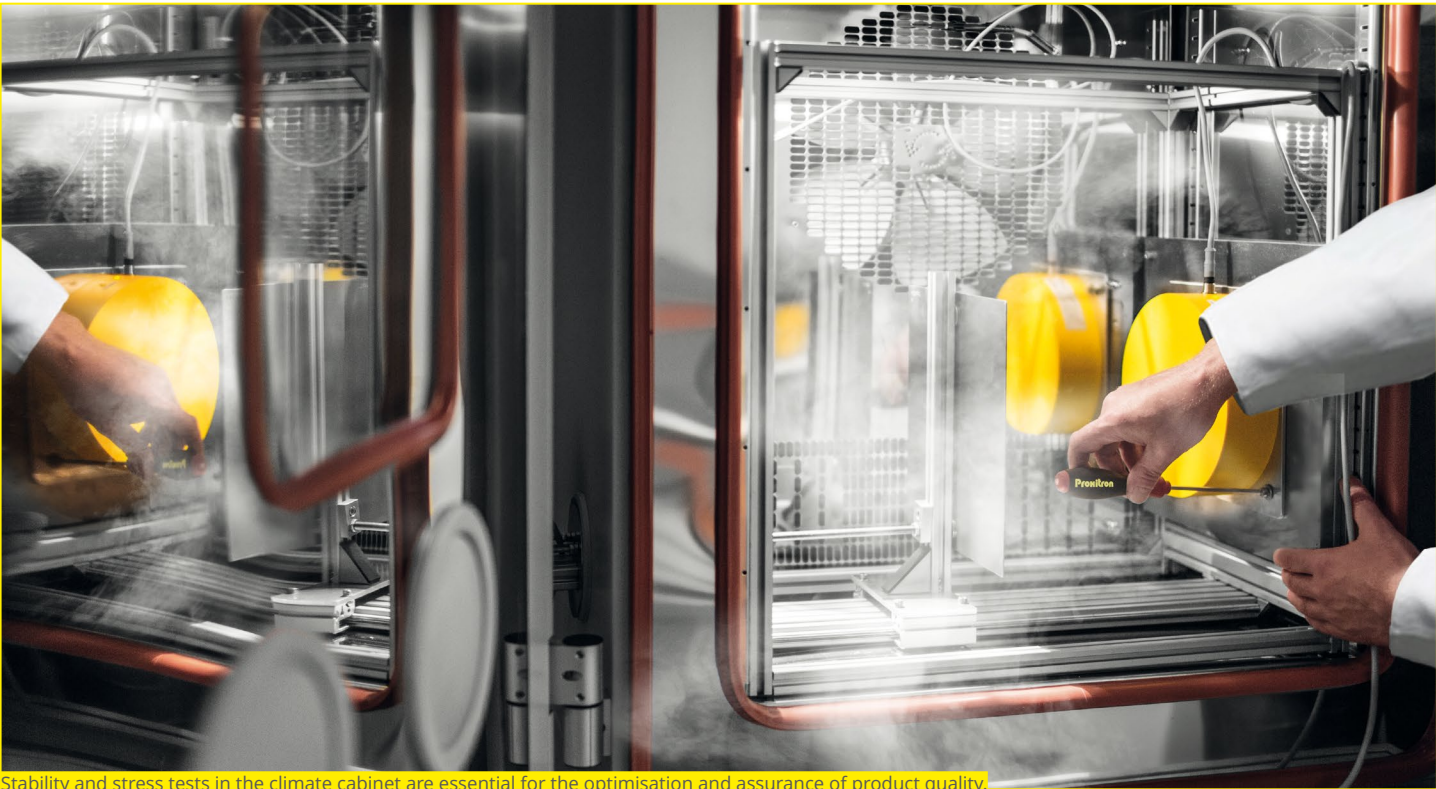
Stability and stress tests in the climate cabinet are essential for the optimisation and assurance of product quality.
