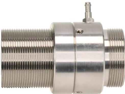
PROXITRON light barriers can be provided with an additional air purge unit DAK 303 to protect the optics from contamination. The recommended operating pressure is 0.15 bar. This value corresponds to a consumption of 60 liters/min. The maximum operating pressure is around 0.3 bar. The scavenging air must be oil-free, dry and dust-free in order to prevent contamination of the optics. For optimal performance of the air-purge unit, the use of an additional protective tube DAK 319 is recommended.
